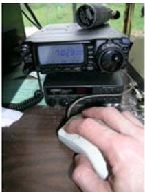
Before closing up the mouse housing, I hooked up my VOM, set it to continuity check and confirmed that I made all my connections correctly. Then I reassembled the mouse housing, and connected to my FT100. Voila, it works great!
